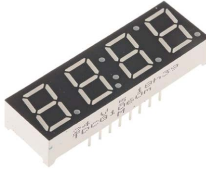
Figure 3.65: 4-digit, multiplexed 7-segment LED display.
