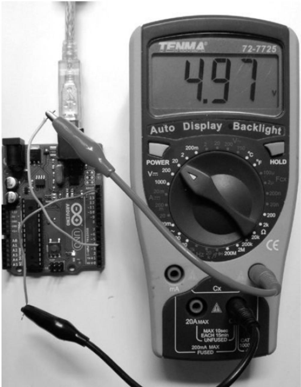
If you don't have enough "D" labeled pins, you can actually use the pins that are labeled "A". Though, the pins labeled "A" are for analog, and you only need to do a little modification by adding **14** to the analog pin number. To do this, simply modify the first line in the above sketch and type pin as **14** instead of **4**. Then move the positive lead of the multimeter to pin A0 on your Arduino Uno.
