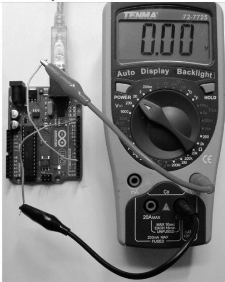
You should set the multimeter to its direct current value of about 0-20V. The negative lead (black) should be joined to the ground pin and the positive lead should be connected to the digital pin at 4 (D4). The wire is connected to the probe and then inserted into the socket headers of your Arduino board.
