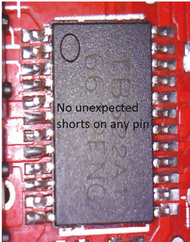
Figure 6-100. Check for any shorts on the H-bridge
