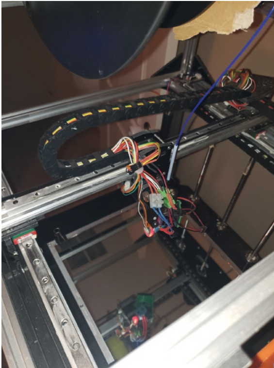
Figure 4-14. FT5 gantry X, Y, and Z axes
