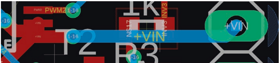
Figure 6-31. Connect the +VIN pin of the H-bridge to the header pin (+VIN)
