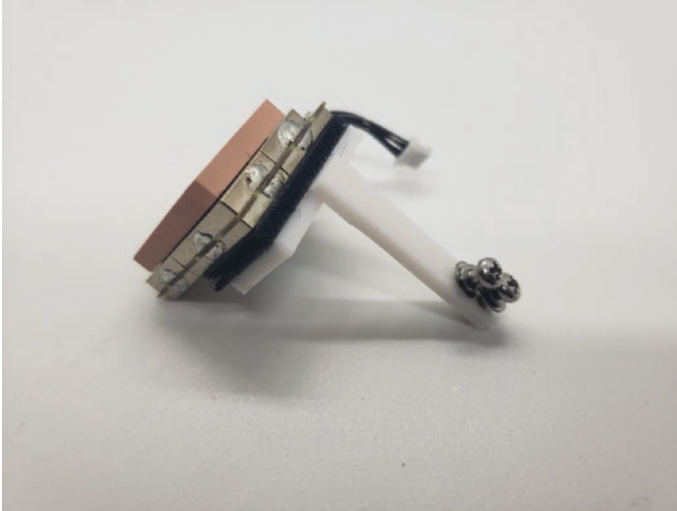
Figure 8-46. Attach the GPS module to the GPS mount using Velcro
