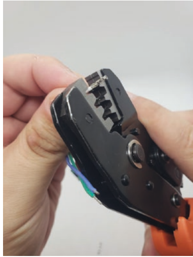
Figure 8-50. Crimp the contact onto the wire
