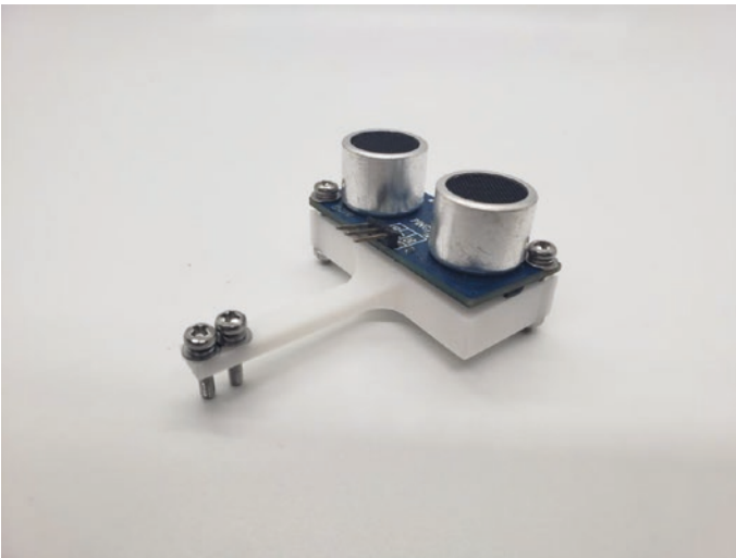
Figure 8-45. Attach the Ultrasonic Sensor to the mount
