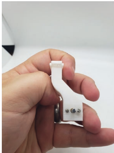
Figure 8-42. Use the M1.6 4mm screws to attach the motor to the wheelbase
