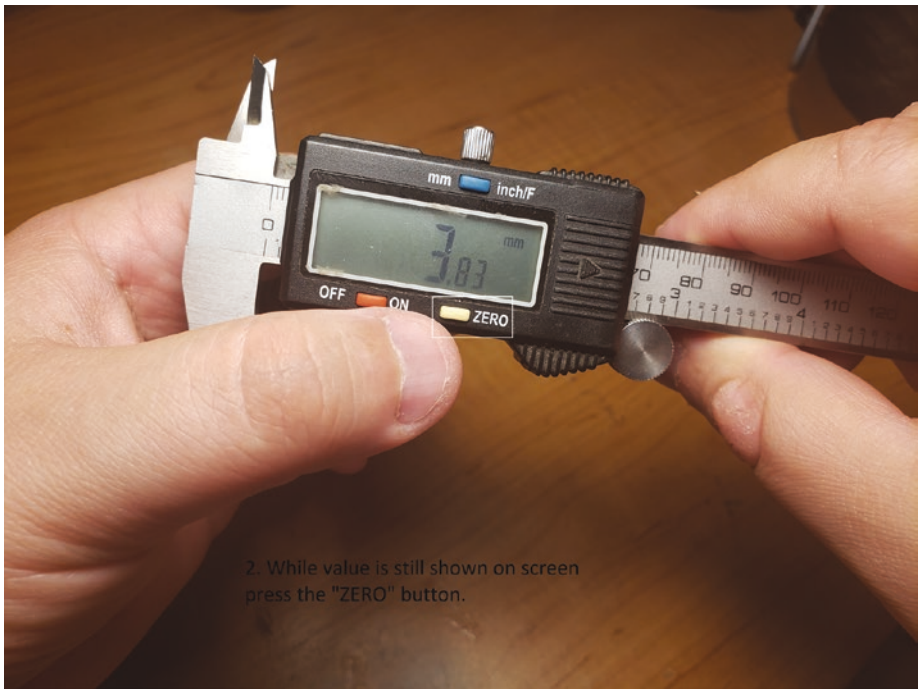
Figure 6-74. Press the zero button without moving the calipers
