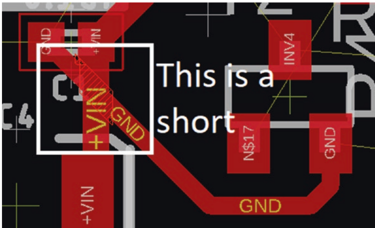
Figure 6-17. This is a short and should always be avoided
