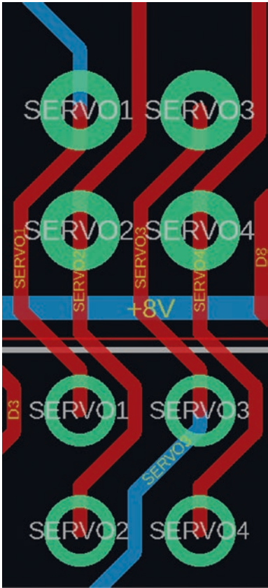
Figure 7-23E. Servo headers connected to the MEGA 2560 Pro
