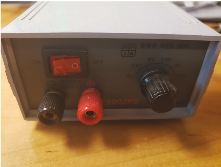
Figure 1-9. Adjustable DC power supply (3, 4.5, 6, 7.5, 9, and 12V)
