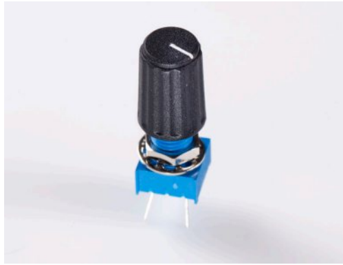
Figure 3-10. Potentiometers can measure rotation
