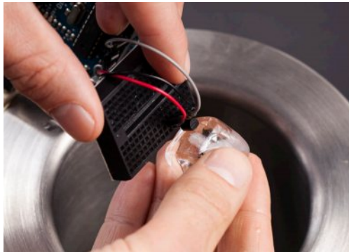
Figure 3-19. Testing the LM35 with an ice cube
