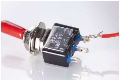
Figure 2-2. Tying a wire to the switch leads
