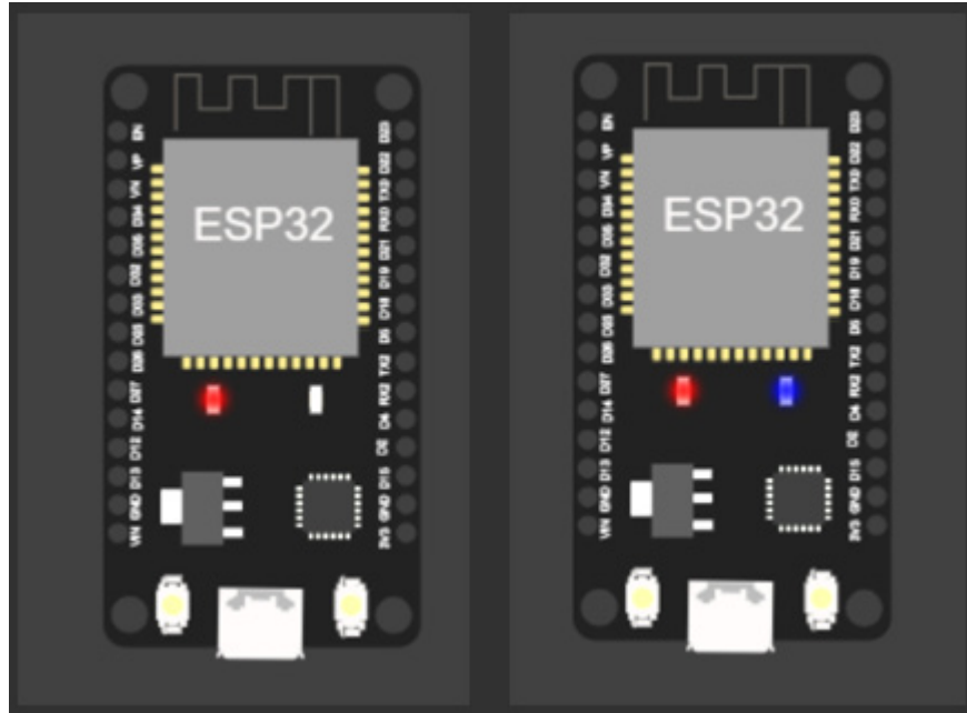
Figure 1.9 – Built-in LED state OFF (left ESP32) and built-in LED state ON (right ESP32)
