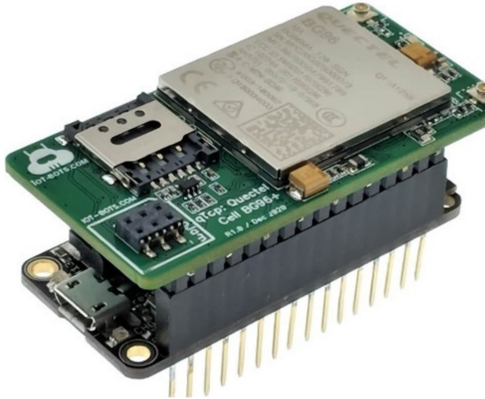
Figure 4.14 – ESP32 connected to a BG95 shield
