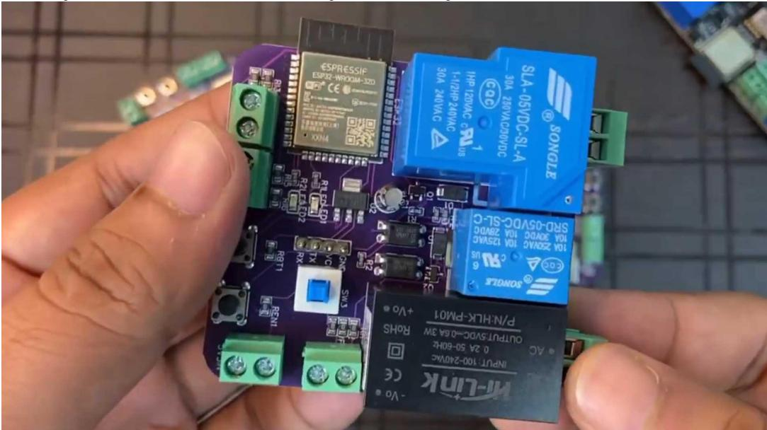
So to solve this problem, I have designed a brand new home automation PCB which can easily handle up to 30 Mpereload. Most of the heavy-load appliances that we use in our homes consume current
