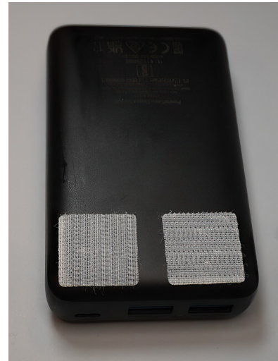
Figure C.2 Power bank with adhesive squares: the squares are attached to the bottom of the power bank.
