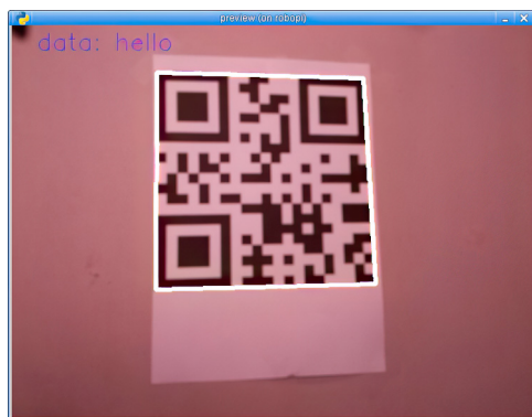
Figure 10.4 Detected QR code: the application draws a box around the detected QR code.
