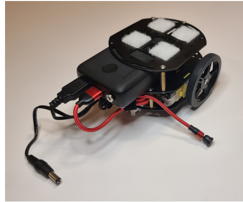
Figure C.4 Chassis with power bank: the Raspberry Pi is placed on the top layer of the chassis.
