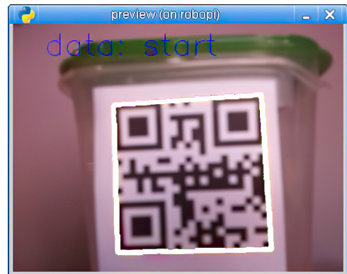
Figure 10.6 Detecting QR codes in live video: detected QR codes are marked on live video.
