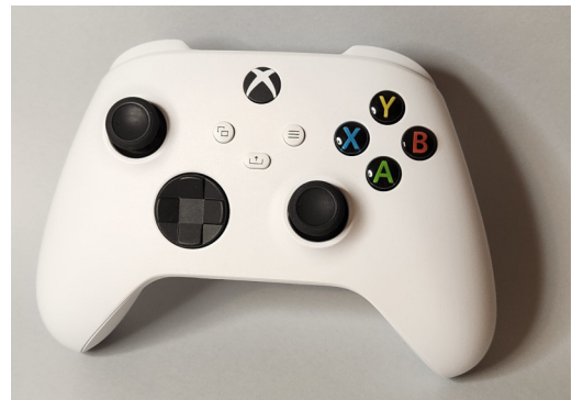
Figure 7.3 Xbox controller: this controller is like the PlayStation controller, but it has two analog sticks.
