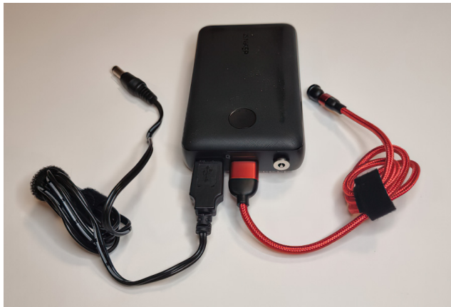
Figure C.3 Power bank with cabling: the USB cable is used to connect power to the Raspberry Pi.
