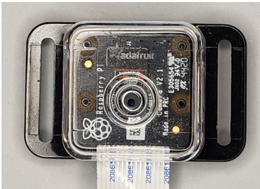
Figure 8.3 Raspberry Pi camera: the camera is enclosed in an Adafruit camera case.
