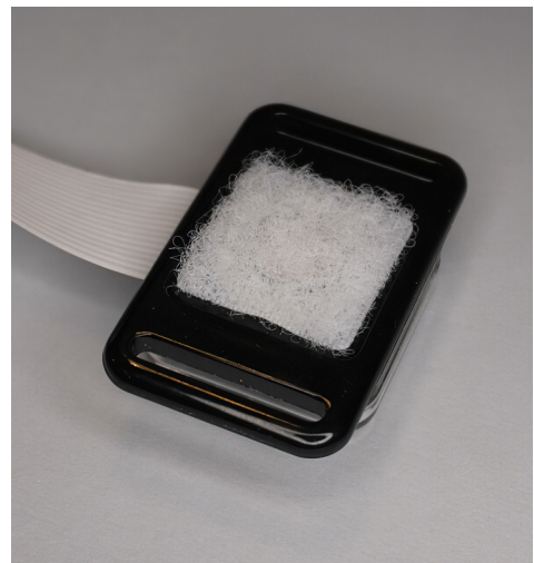
Figure C.7 Camera case: the Velcro squares are attached to the back of the camera case.
