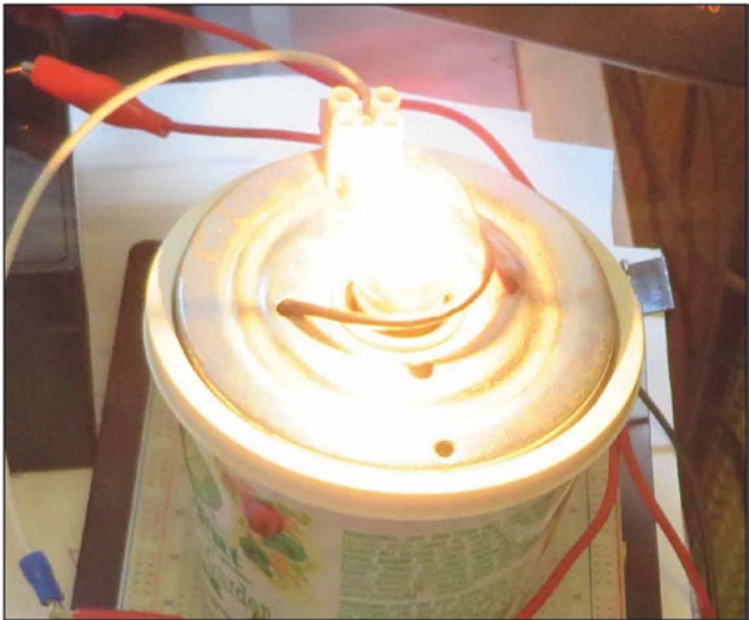
Figure 7-9. Incandescent Bulb Load for PWM at High DC Power
