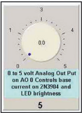
Figure 7-5. Base Current and LED Intensity Rotating Control Knob with Instruction Panel
