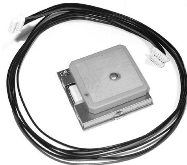
Figure 13-3: A long GPS-receiver-to-shield cable
