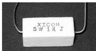
Figure 3-5: A 5-watt resistor
