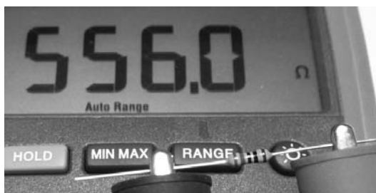
Figure 3-4: Multimeter measuring a 560-ohm 1 percent tolerance resistor
