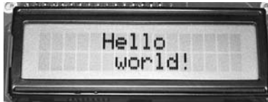
Figure 7-3: LCD demonstration: "Hello world!"
