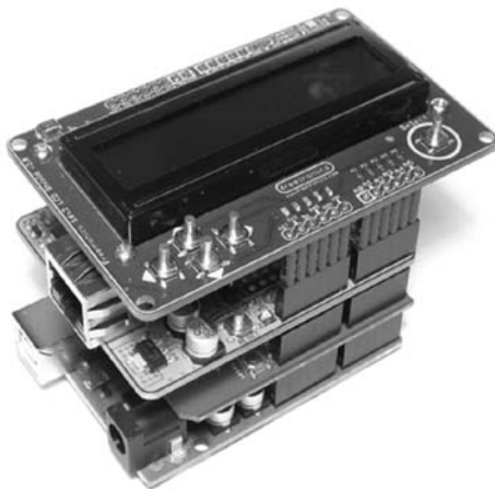
Figure 8-4: Three stacked shields with an Arduino Uno
