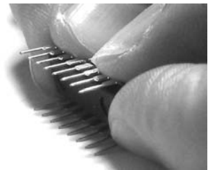
Figure 11-12: Bending the microcontroller pins
