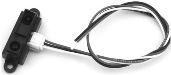
Figure 12-23: The Sharp IR sensor
