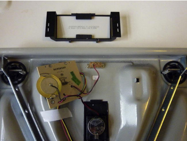
Figure 10-2. Scale after removing the cover and LCD
