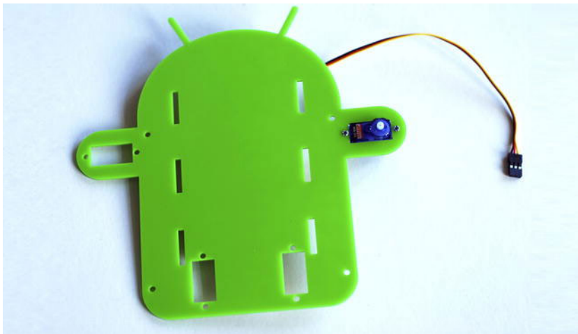
Figure 6-8. Assembling servos to the back body
