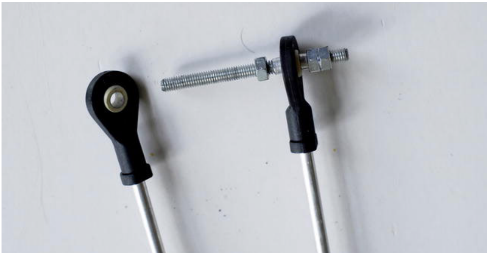
Figure 13-4. Ball joint assembly
