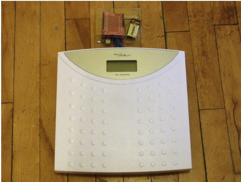
Figure 10-9. Scale finished and plugged to the Arduino and XBee module
