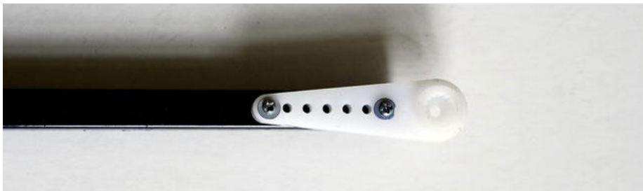
Figure 13-2. Thigh connected to the servo horn
