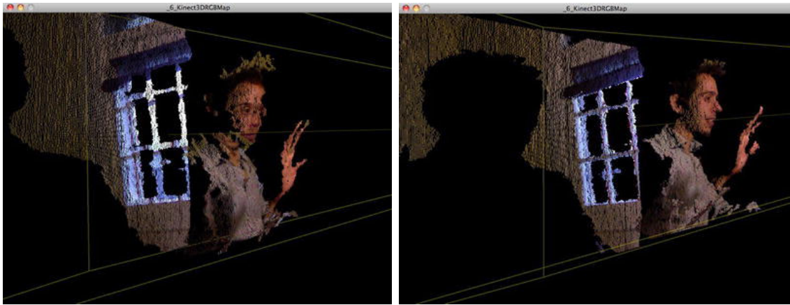
Figure 3-11. RGB image on non-calibrated point cloud (left) and calibrated point cloud (right)
