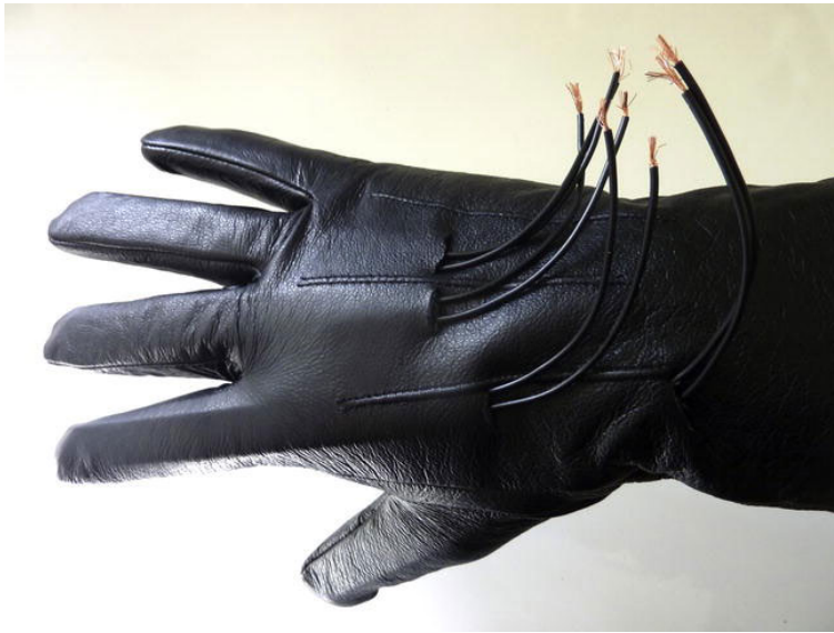
Figure 11-7. Flex sensors installed in the glove
