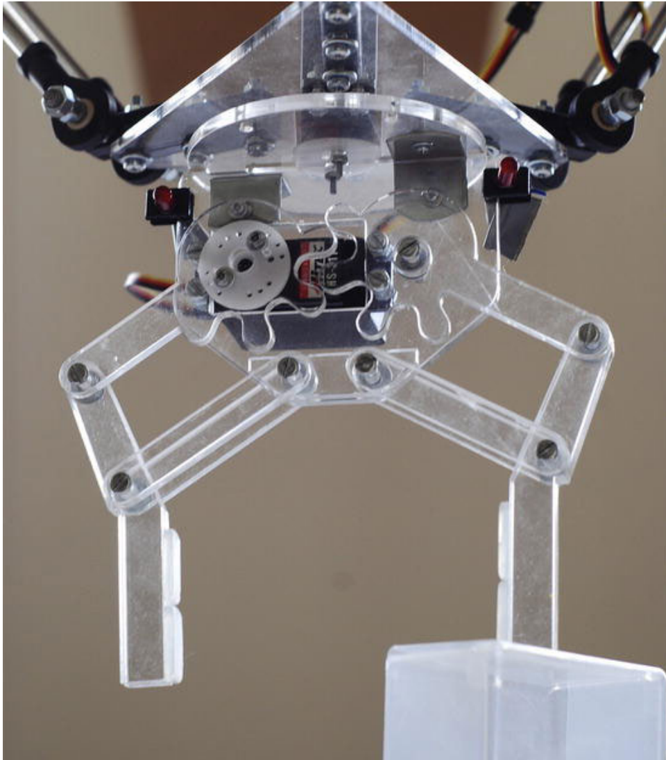
Figure 13-15. Assembled gripper with servo and LEDs on board
