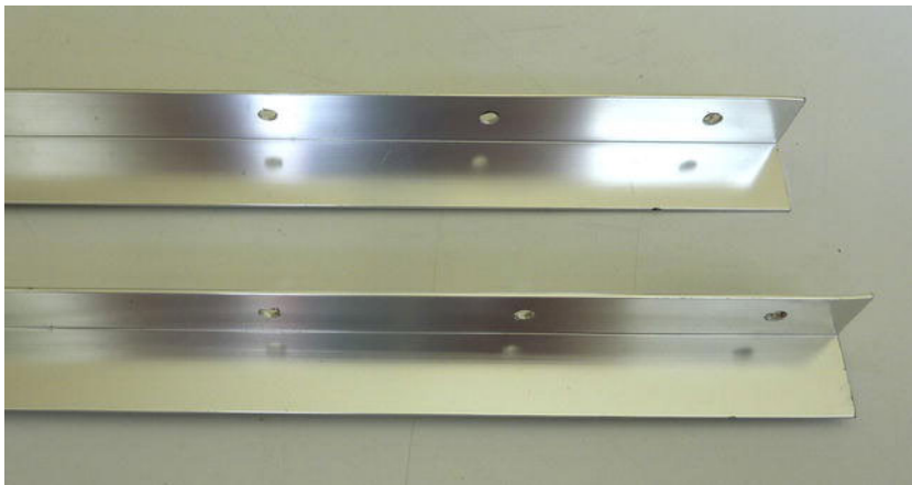
Figure 12-13. Bracing aluminum angles after drilling the holes
