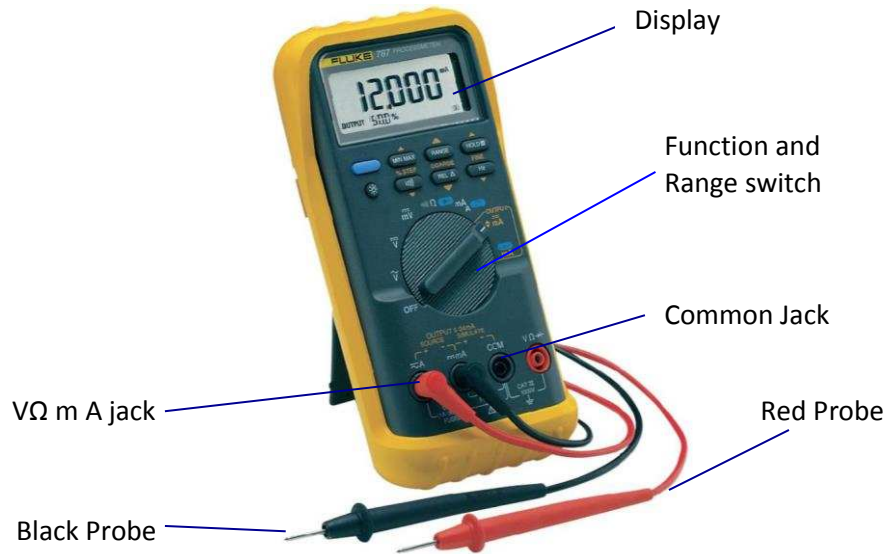
Figure 29: Parts of a multimeter
