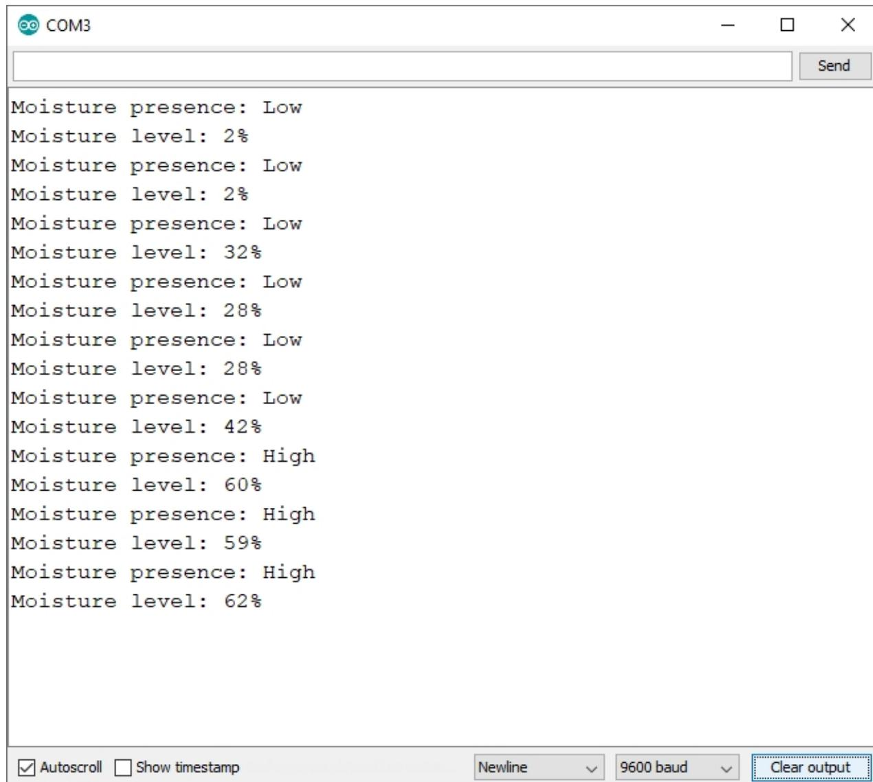
The screenshot shows the Arduino Serial Monitor window titled "COM3". The window displays a series of moisture sensor readings. The data is as follows:
