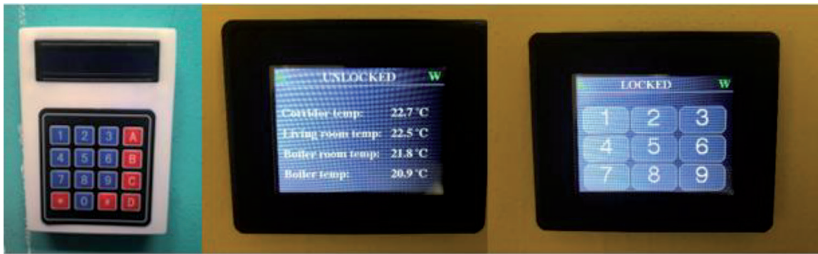
Figure 2. Input board in boiler room.
