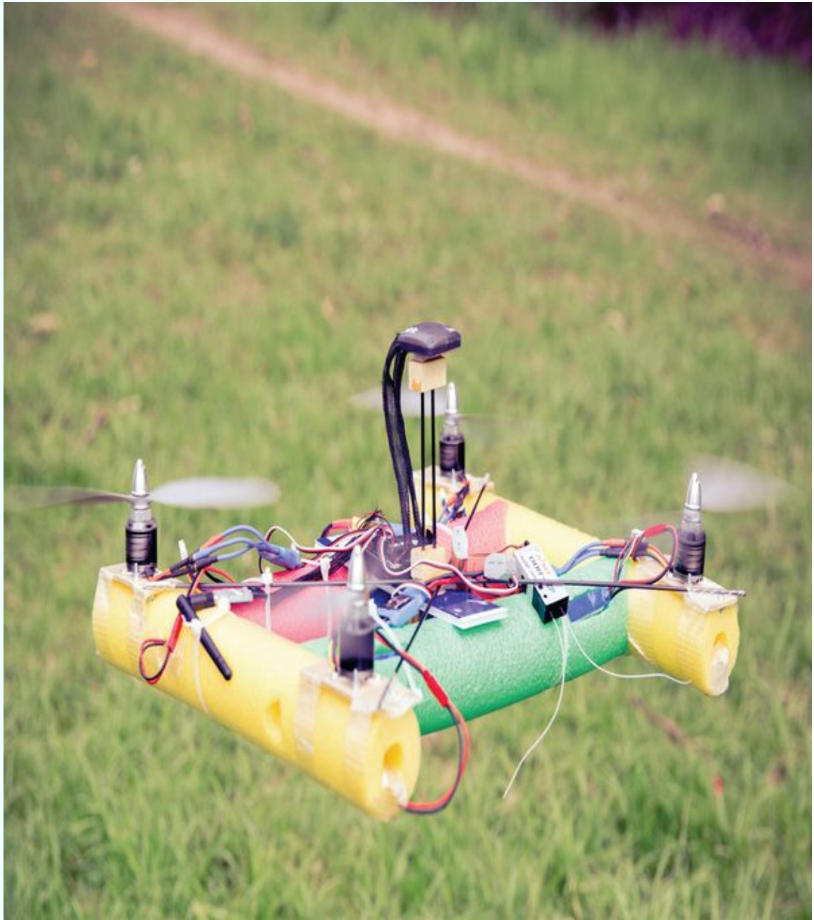
Figure 10-1. Structural supports for this drone are made from styrofoal pool noodles
