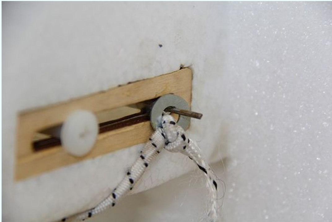
Figure 13-3. The bungee secures to the pin of the drop mechanism; the servo retracts the pin to release the bungee and drop the payload
