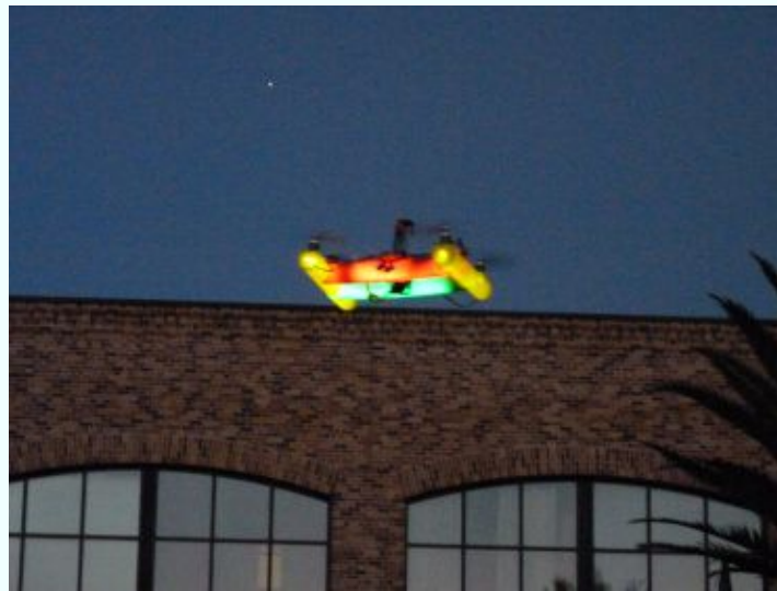
Figure 10-2. Pool noodle copter lit up with internal LEDs
