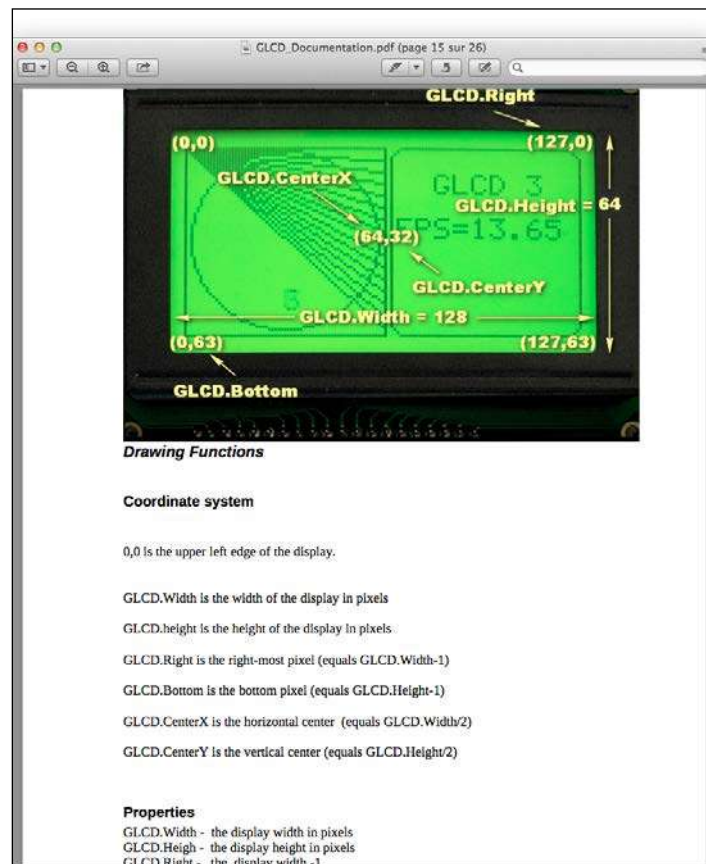
The documentation of gLCD-Arduino showing the screen coordinates system
